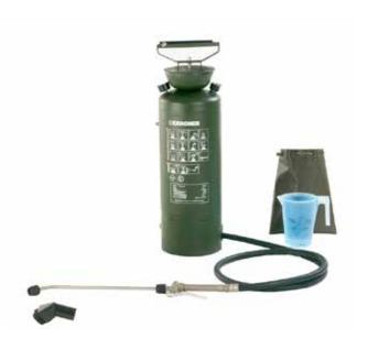
With an operating pressure of up to 6 bar, the DS 10 mixes decontamination or cleaning agents with its integrated mixer unit, then emits fine quantities of spray through a stainless steel nozzle.
